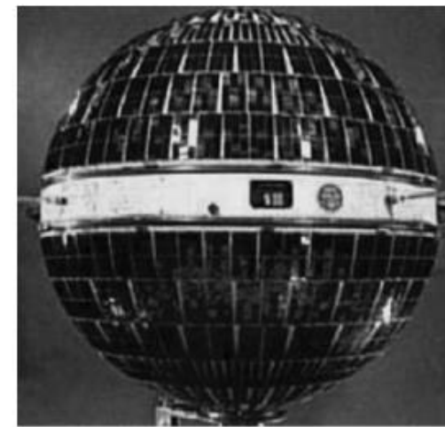
Figure 1.12 Courier-1B (Courtesy: US Army)
